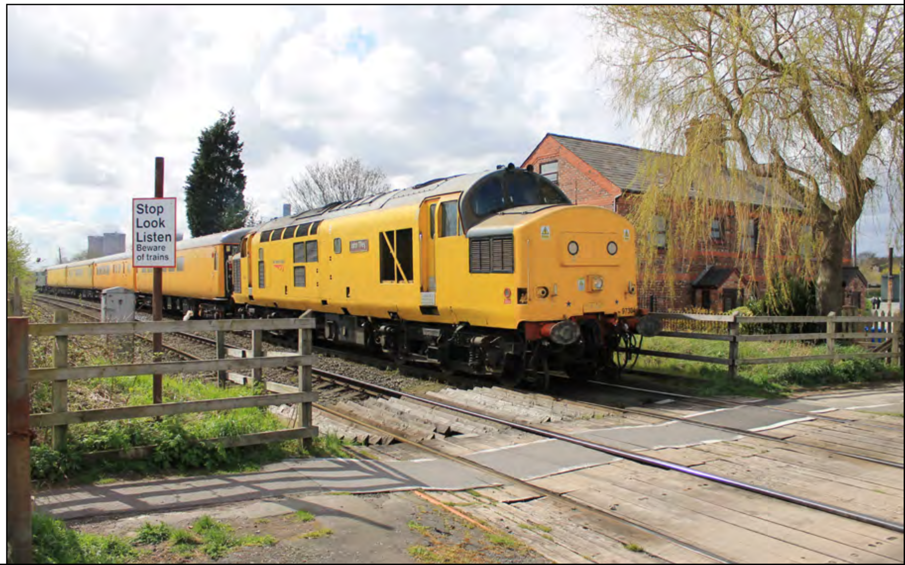
Below: On April 25th, Class 97 304 (with 31 106 on the rear) heads the 1Q13 test train running from Derby - Edinburgh - Derby, seen here passing through Farrington Jct., crossing from the fast to slow line. Michael Lynam
