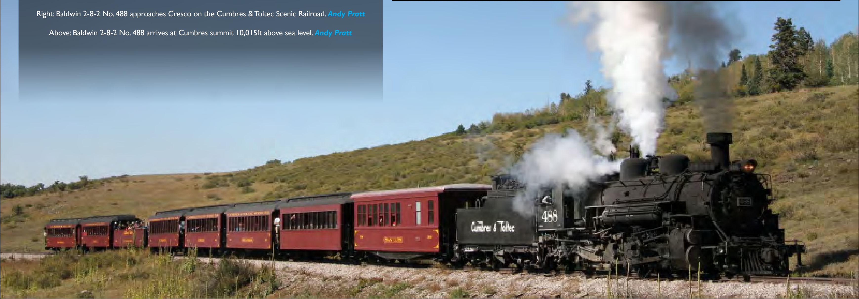
Main: The 64 mile long 3ft Gauge Cumbres & Toltec Scenic Railroad operates from Chama, New Mexico to Antonito, Colorado. Here 1925 Baldwin built K-36 2-8-2 No. 488 approaches a level crossing with State Road 17 between Chama and Cumbres. Andy Pratt
