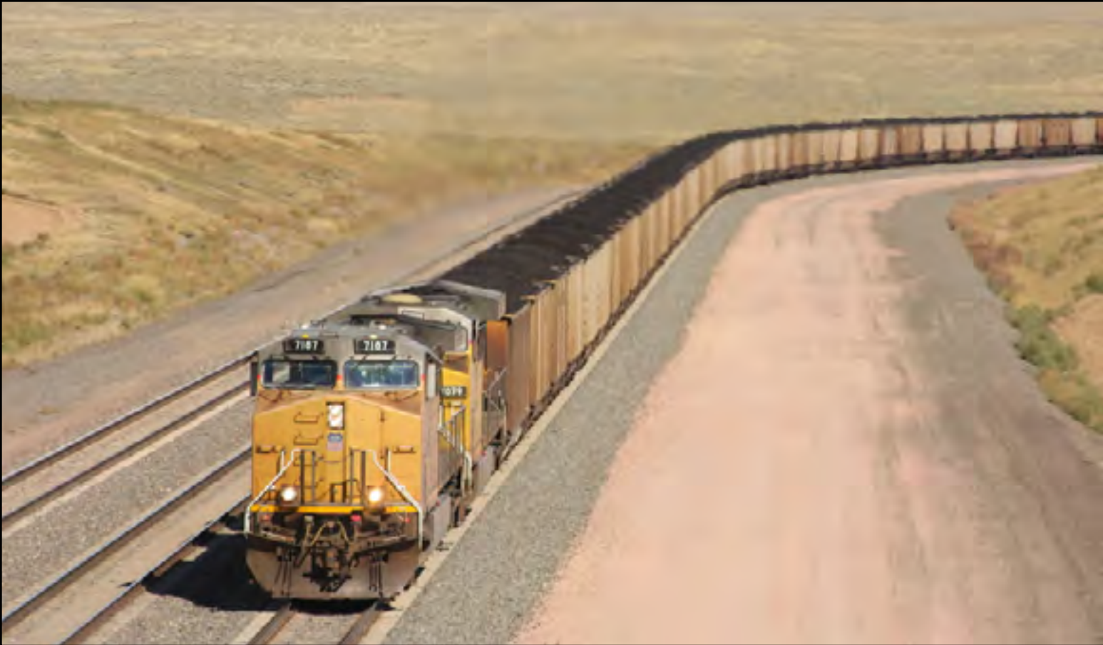
Above: In the Powder River Coal Basin now, viewed from the Walker Creek Road Bridge, a Union Pacific loaded coal train heads south from the Powder River Coalfield towards Shawnee Jct., Wyoming. The layout here is 3 tracks wide with all 3 tracks being bidirectional. Andy Pratt
