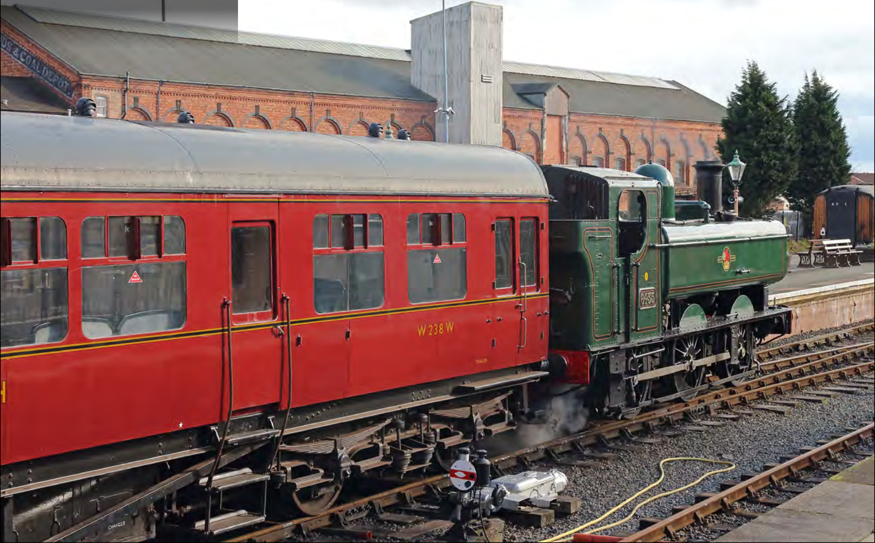
Great Western Railway 6400 Class 0-6-0 pannier tank No. 6435, is seen at Kidderminster working the single coach 'Autotrain' Class47
