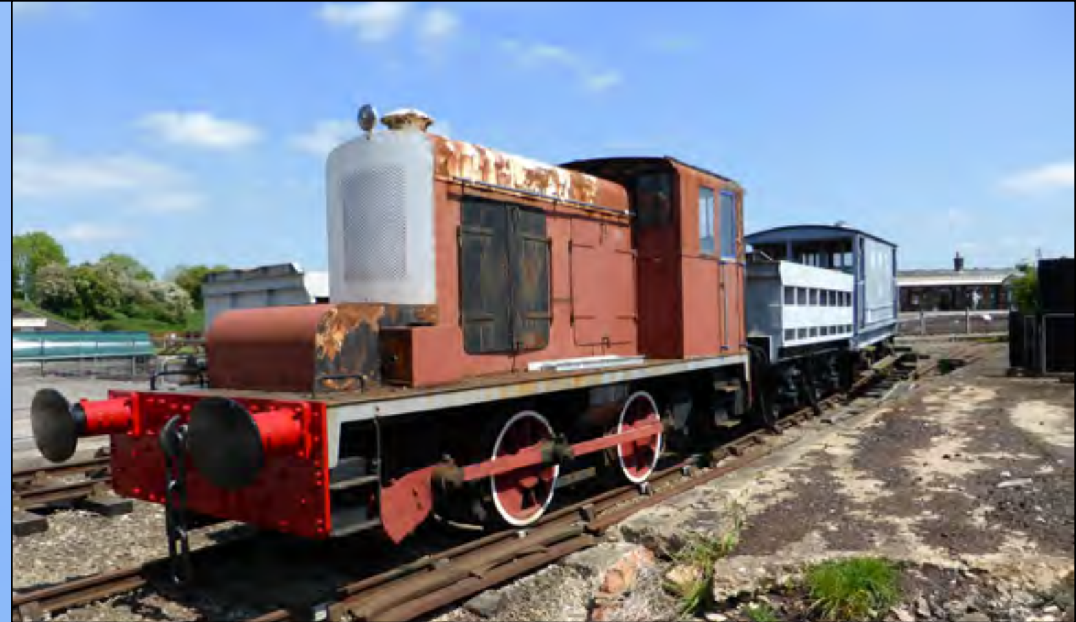
Above: Hibberd 0-4-0DM No. 3271 'Walrus' is seen out of use at Quainton Road. The loco has minor engine problems and worn tyres. Andrew Wilson
