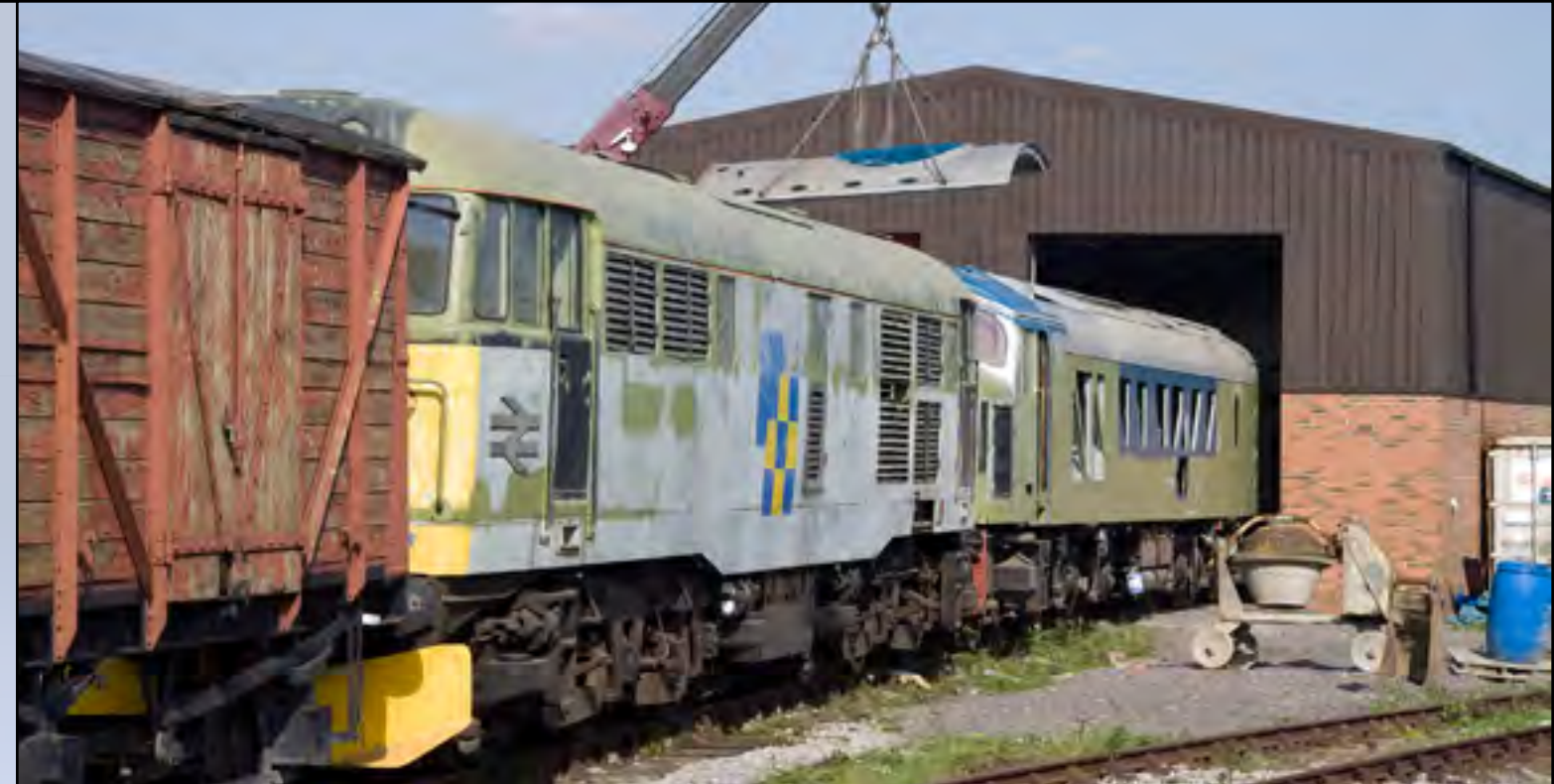
Above: Part way through repaint, Class 46 045 has its roof lowered back into place, whilst 31 271 also looks like it is getting attention from the paint pot. Richard Hargreaves
