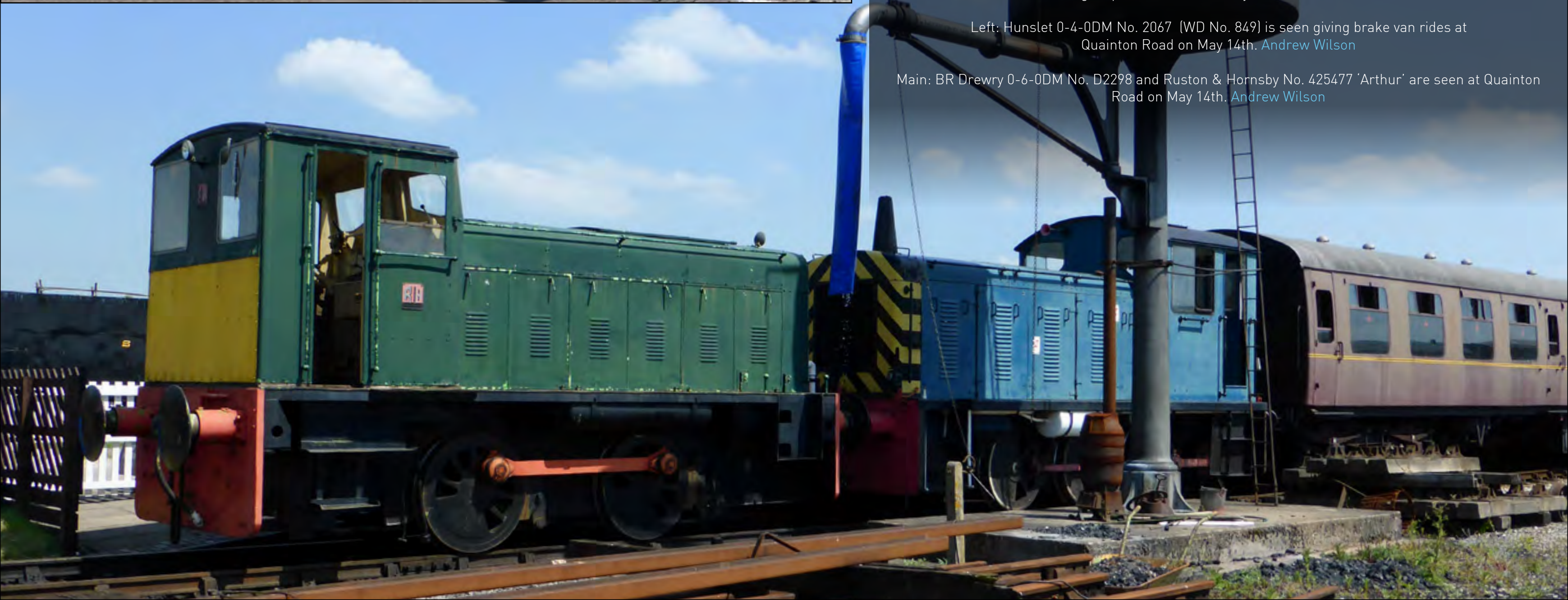
Above: Hibberd 0-4-0DM No. 3271 'Walrus' is seen out of use at Quainton Road. The loco has minor engine problems and worn tyres. Andrew Wilson
