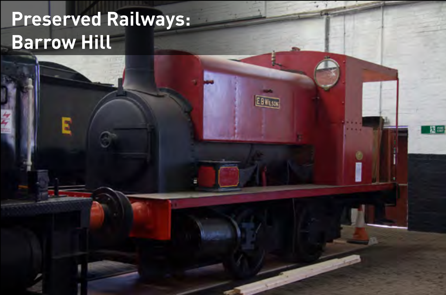
Above: Manning Wardle 0-4-0 No. 1795 'E B WILSON' is pictured under restoration inside the roundhouse on May 3rd. Richard Hargreaves
