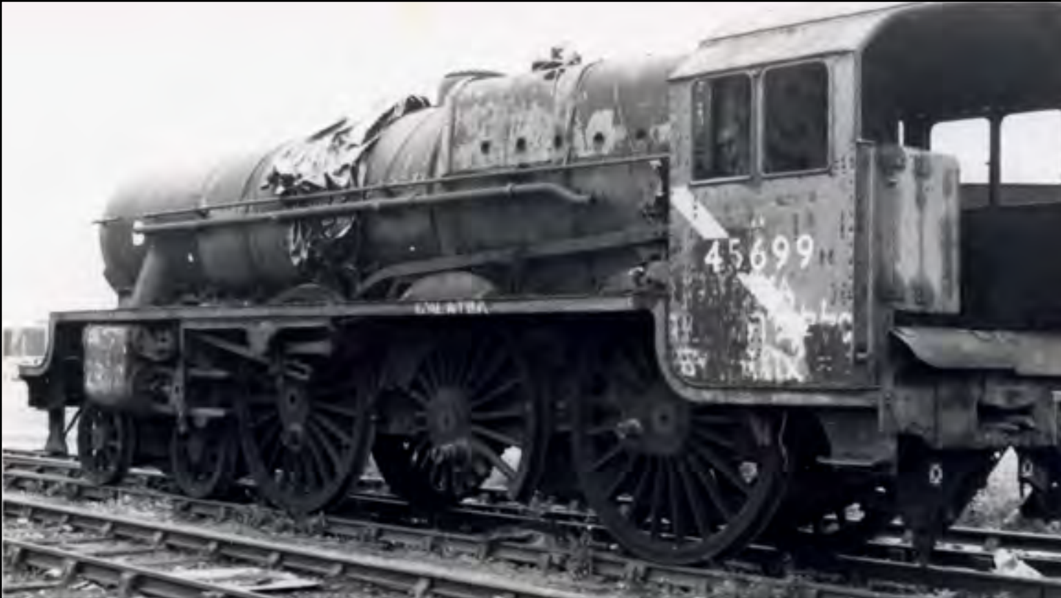
Above: Stanier Jubilee 4-6-0 No. 45699 'Galatea' is seen in scrap condition with broken centre wheel at Barry Island on August 19th 1979. Steve Stepney
